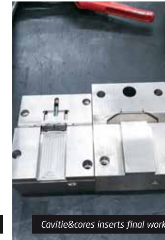
Cavities&cores inserts final works
