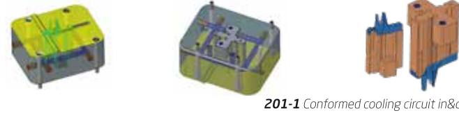
201-1 Conformed cooling circuit in&out
