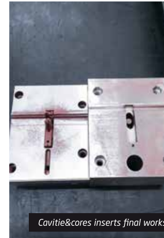
Cavities&cores inserts final works
