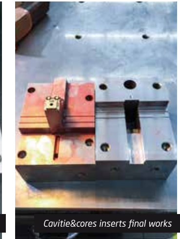
Cavities&cores inserts final works
